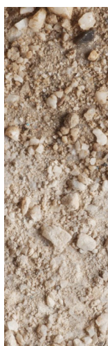
Halfverharding type: 'Stabilizer', 'Maasmix'
