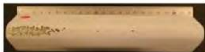
Figure 4. Blade sample with polyester gelcoat, tested at 123-157ms -1 , 30-35mm/h simulated rain for 60 minutes. Source: [11].
