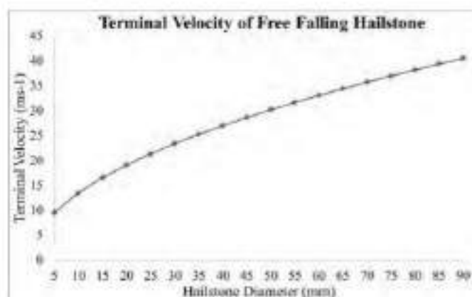
Figure 23. Terminal velocity diameter, according to equation [68], for an air density of 1.29\text{kgm}^{-3} and a drag coefficient of 0.5.
