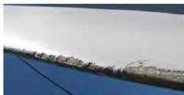
Figure 3. Example of leading edge erosion. Source: [14]
