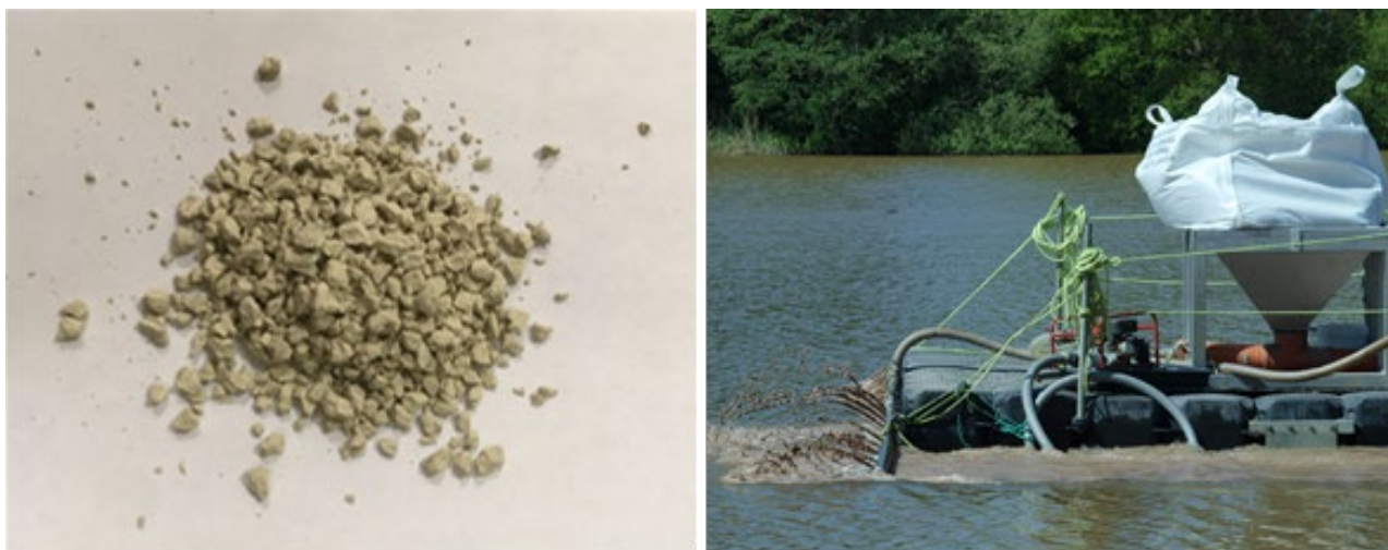
Figure 1. On the left, a picture of Phoslock® as a dry material and on the right Phoslock® being mixed with lake water and applied on the surface of Lake de Kuil (the Netherlands).
