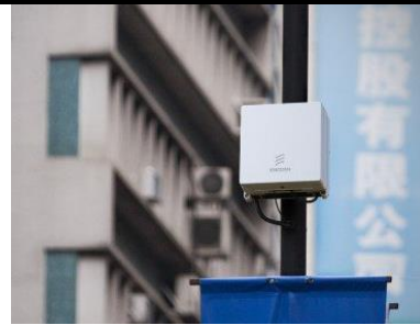
Figuur 6: Outdoor: Ericsson Radio 2203 (200x200x100mm)
