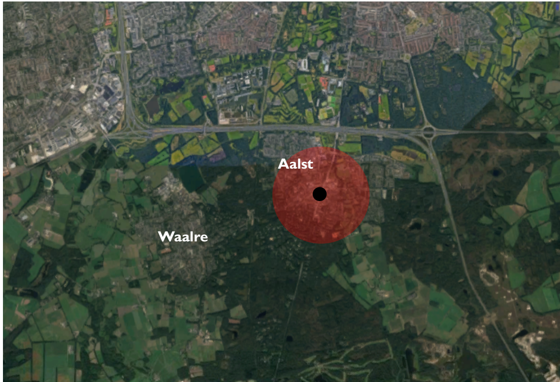
Area of influence of the HOV stop when walking to the stop (800 meters) source: google maps, edited by the authors
