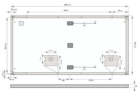
Measurements in mm
